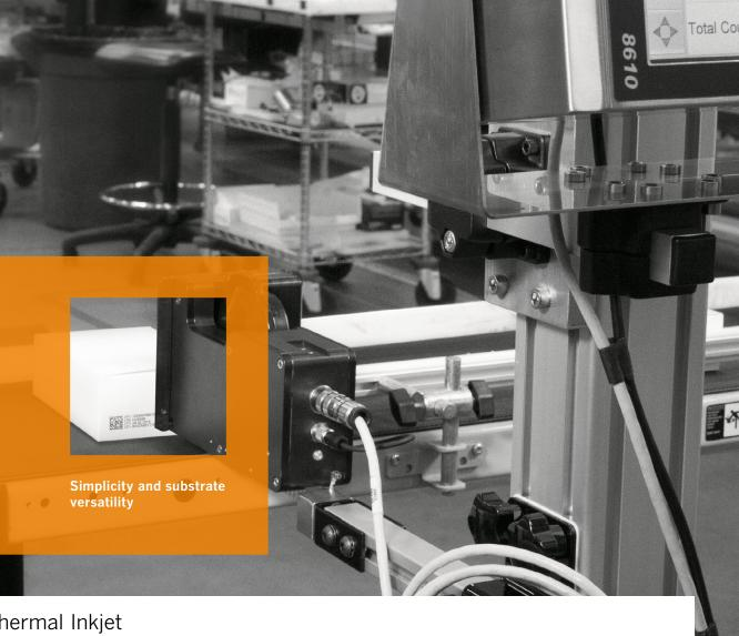
Revolutionizing thermal inkjet technology, the Videojet 8610 combines the simplicity of a cartridge-based printing system with MEK-based, industrial ink performance for non-porous substrates.
